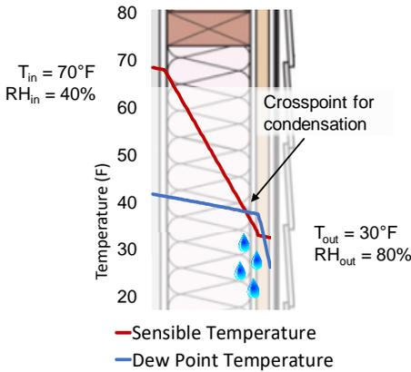
In a cold climate, the indoor vapor content is typically higher, and thus vapor moves outwards. Figure 2 depicts a scenario for which condensation occurs inside the wall due to the lack of an interior vapor retarder. The red line represents how temperature is distributed inside the wall. The blue line illustrates the dew-point temperature. As seen in the figure, when the temperature drops below dew-point, condensation occurs.
