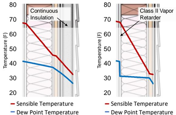
**Figure 3:** Intermediate condensation can be avoided for walls in cold climates by either make them warmer (left), or install an interior vapor retarder (right)
