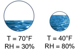
**Figure 1:** Humid air seen as spheres. Their size and vapor capacity depend on temperature, but both spheres contain an equal amount of vapor.
