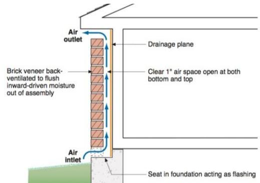
Figure 3: Back ventilation for brick veneer walls.
