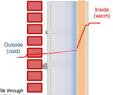
Figure 1: Temperature profile through an internally insulated CMU wall
