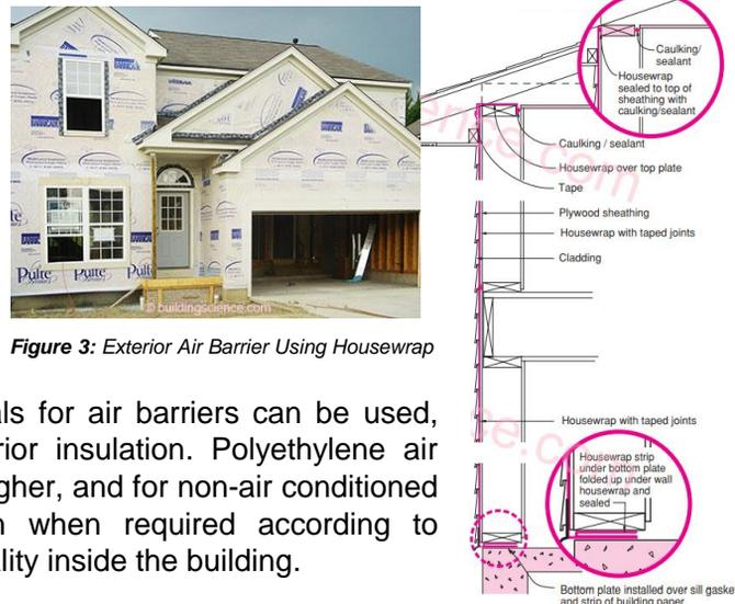
Figure 3: Exterior Air Barrier Using Housewrap
