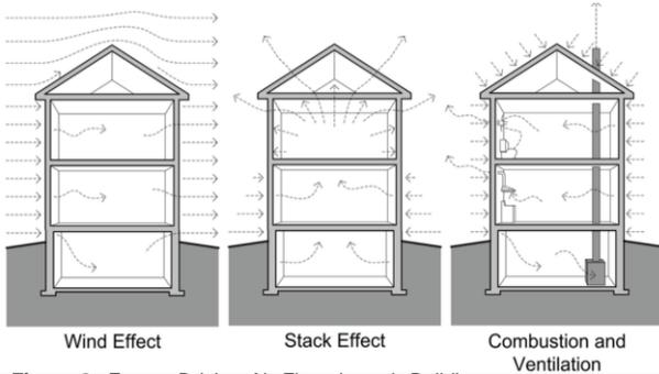
Figure 2: Forces Driving Air Flow through Building Enclosure
